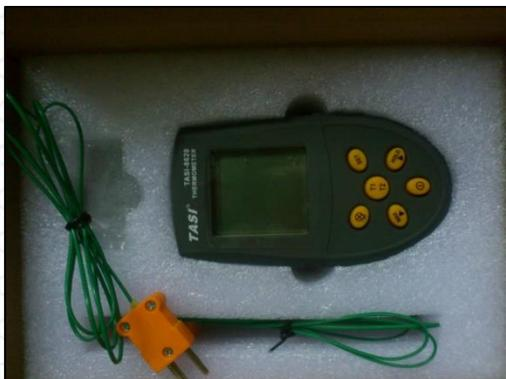
Gambar 3.5 *Thermocouple*
