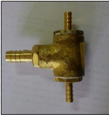
Gambar 3.3 Skema *Mixing chamber*
