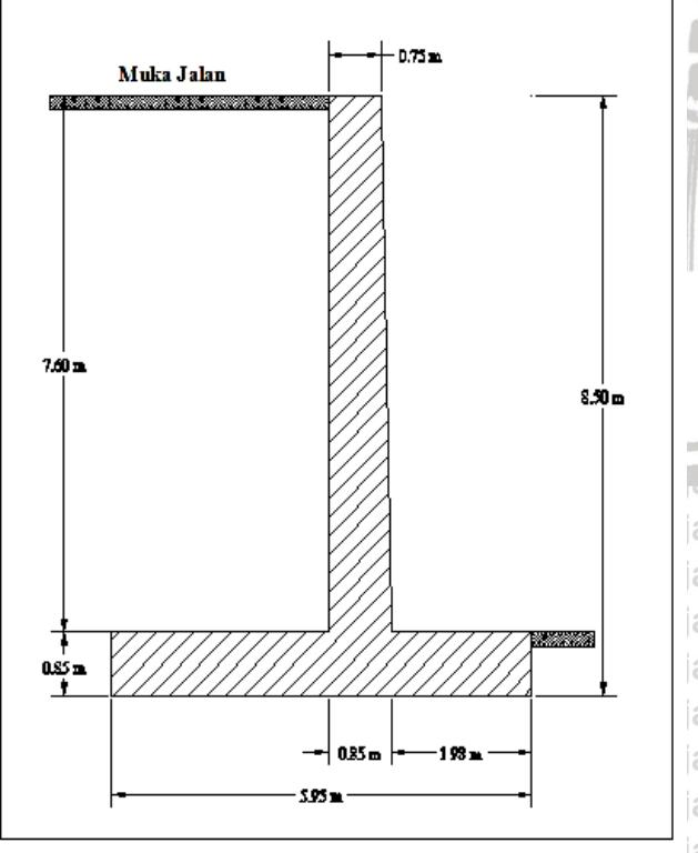
Gambar 4.43. Dimensi Dinding Penahan Tanah Kantilever
