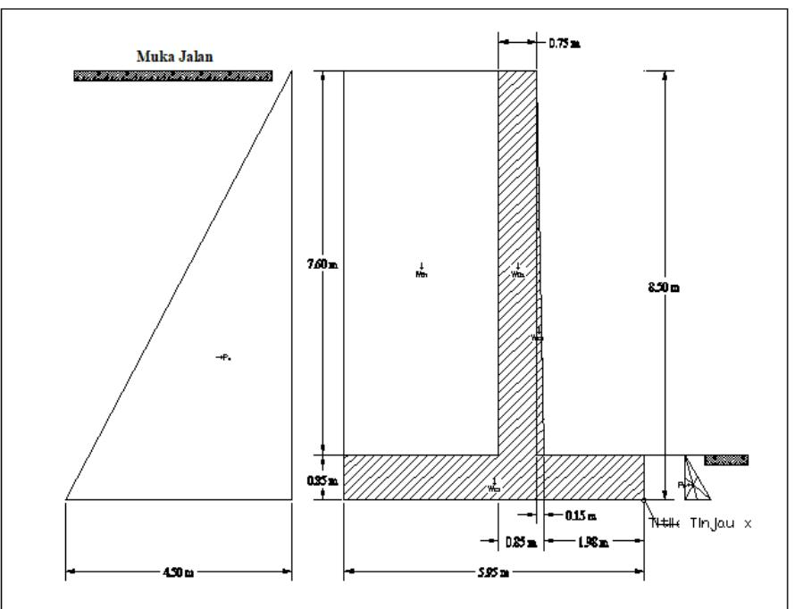
*Gambar 4.44.* Diagram Gaya-gaya Pada Dinding Penahan Tanah Kantilever
