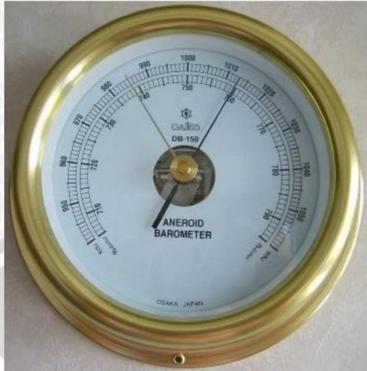
Gambar 6. Barometer
