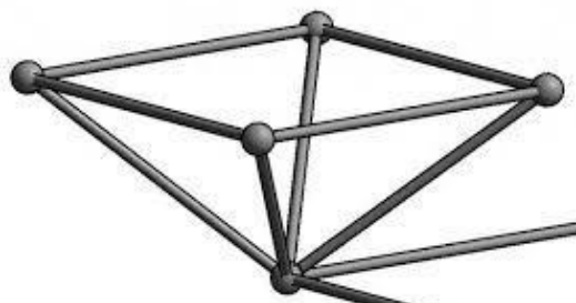
Gambar 4.69 Modul Space Frame Tetrahedron sumber: googleimage.com
