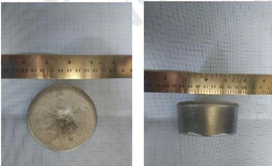
Gambar 3.8 *Ingot* Al-Mg-Si
