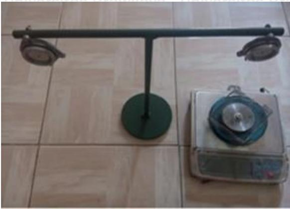
Gambar 3.7 Alat Uji Piknometri
