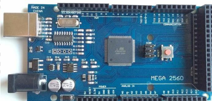
**Gambar 2.1 Arduino Mega 2560**
