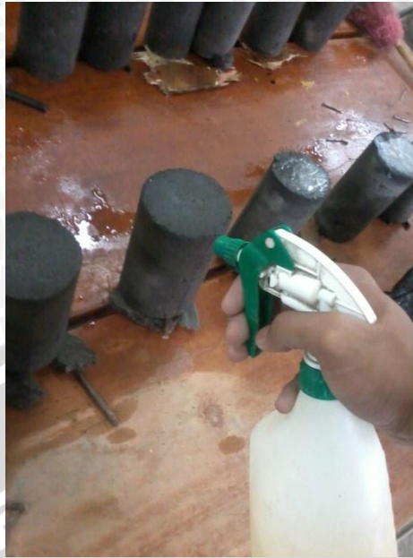
Curing Benda Uji Pull Out
