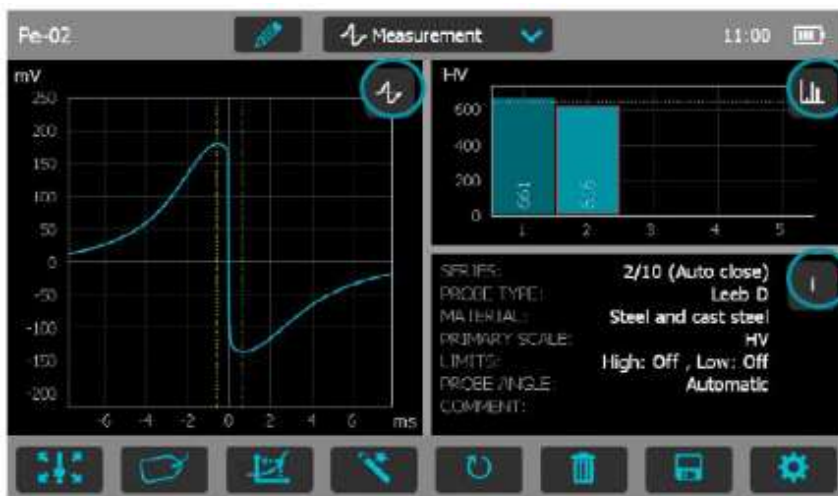
Gambar 2.10 Measurement and Statistic View pada Equotip
