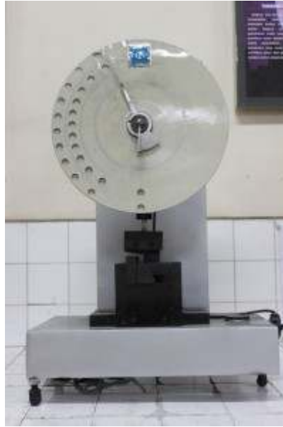
Gambar 3.6 Charpy Impact Non – Ferrous
