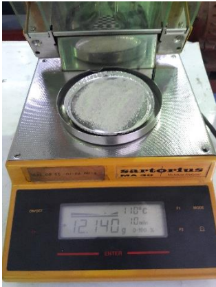
Proses pengujian kadar air zeolit
