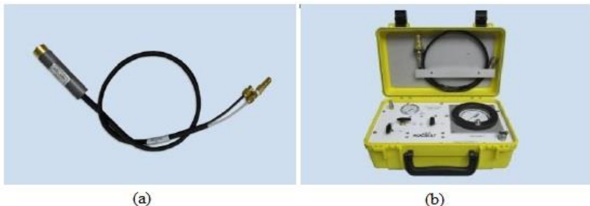
Gambar 2.16 (a) material Pneumatic Piezometer (b) alat monitoring Pneumatic Piezometer sumber: PT. Teknindo Geosistem Unggul
