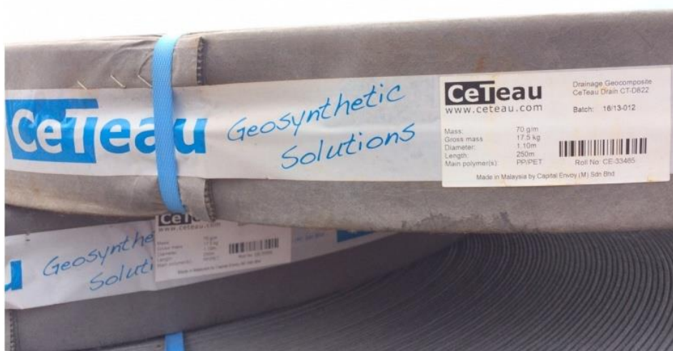
Gambar 4.2 Vertical drains tipe CeTeau Drain CT-D822
