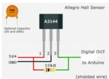
Gambar 3.7 Skematik sensor hall effect A3144
