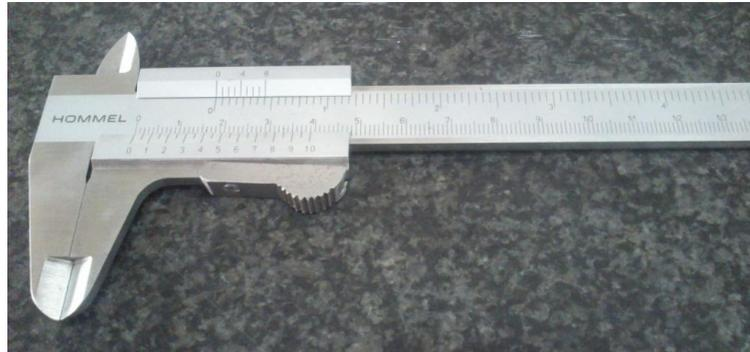
Gambar 3.2 *Vernier Caliper*
