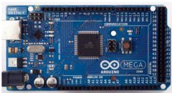
Gambar 2. 7 Arduino mega 2560
