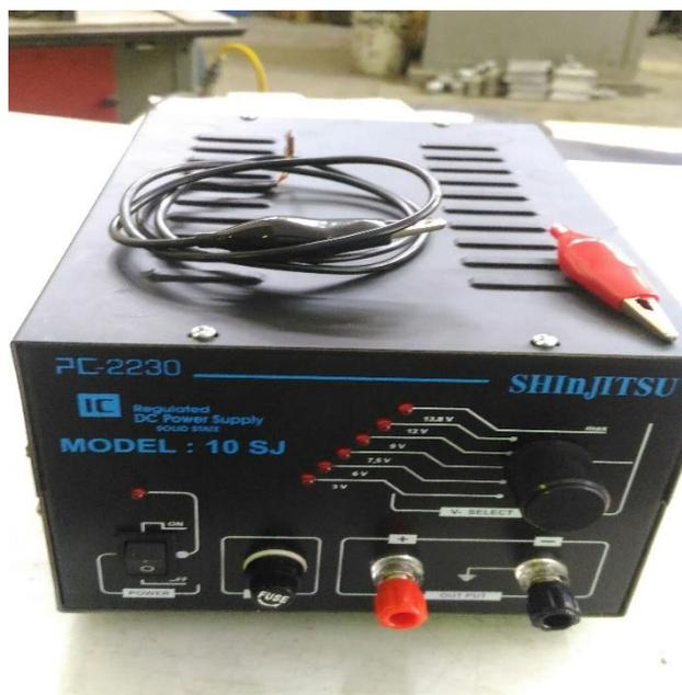
Gambar 3.1 *Regulated DC Power Supply 10 SJ*
