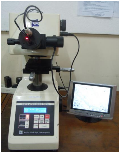
Gambar 3.5 Digital micro vickers hardness tester TH712
