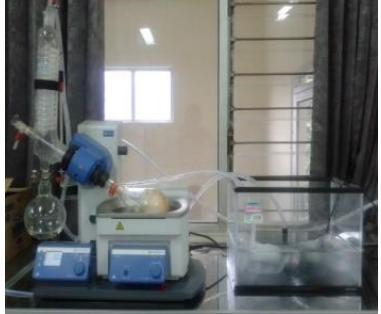
A photograph of a rotary evaporator machine connected to a vacuum system for sample drying.                                                                                      |
