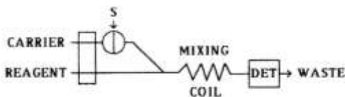
Gambar 2.2 Susunan Komponen Dasar FIA. S = sampel injection, DET = Detektor [35]
