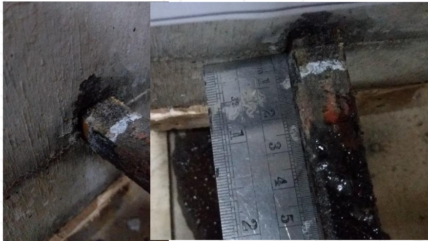
Gambar Keruntuhan Benda Uji Pull Out A 0 B 1 – 3
