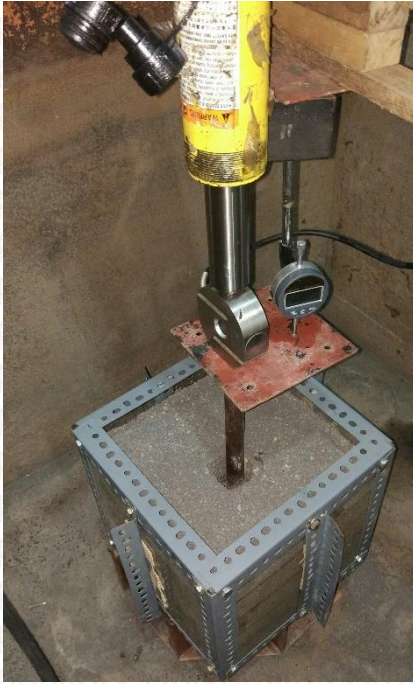
Gambar Uji Pembebanan (load test)
