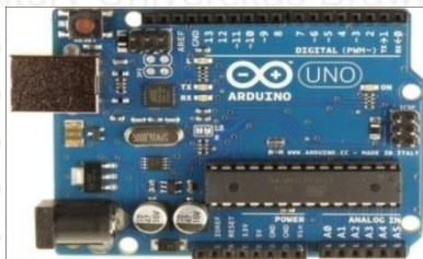
Gambar 2. 25 Board Arduino Uno berbasis ATmega 328P
