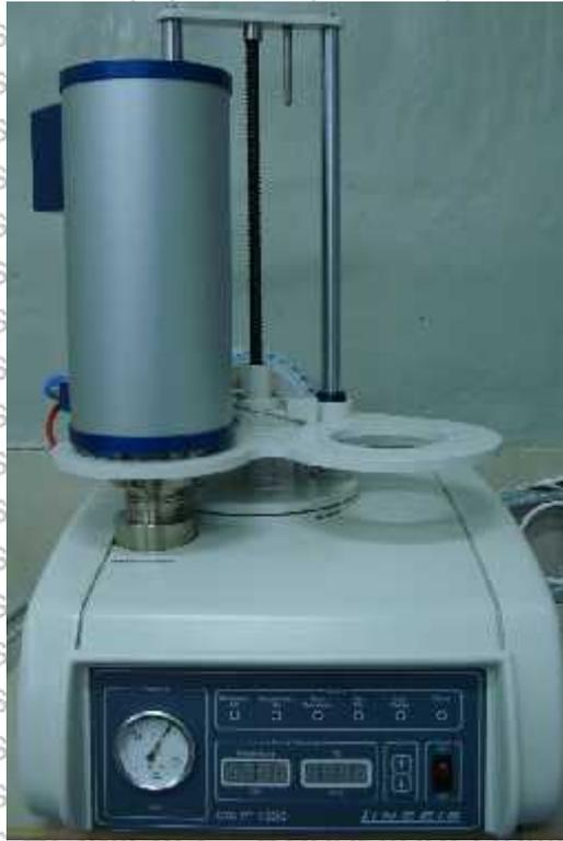
Gambar 4.2 Alat uji STA PT 1600 LINSEIS
