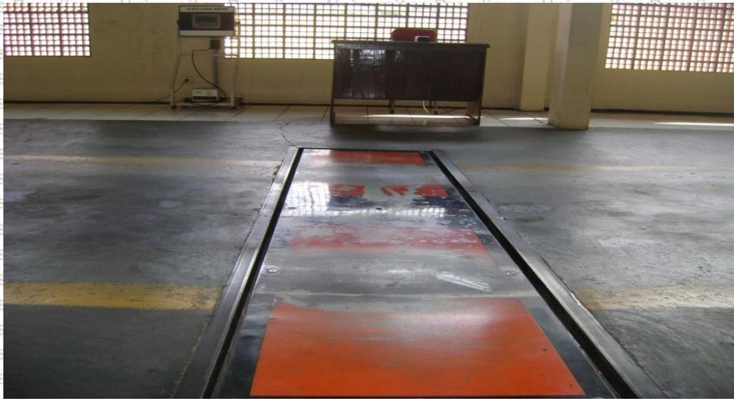
Gambar 5.8 Alat Axie Load Meter
