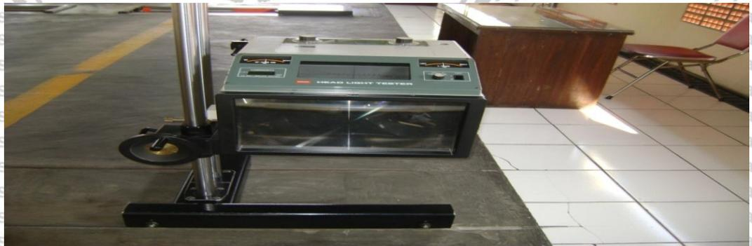
Gambar 5.6 Alat *Head Light Tester*
