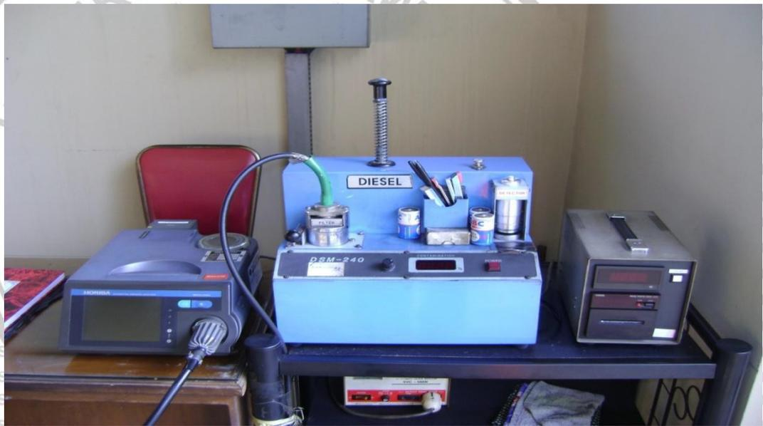
Gambar 5.1 CO/HC Analyzer Diesel Smoke
