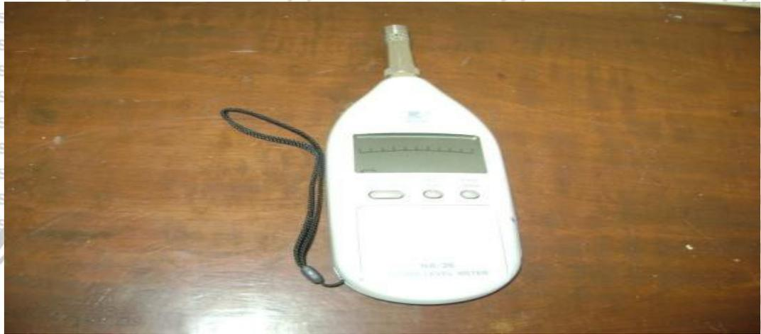
Gambar 5.5 Alat *Sound Level Meter*
