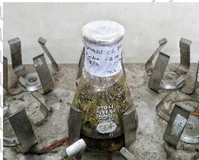
Proses maserasi dan penggojokan larutan sampel menggunakan *orbital shaker*
