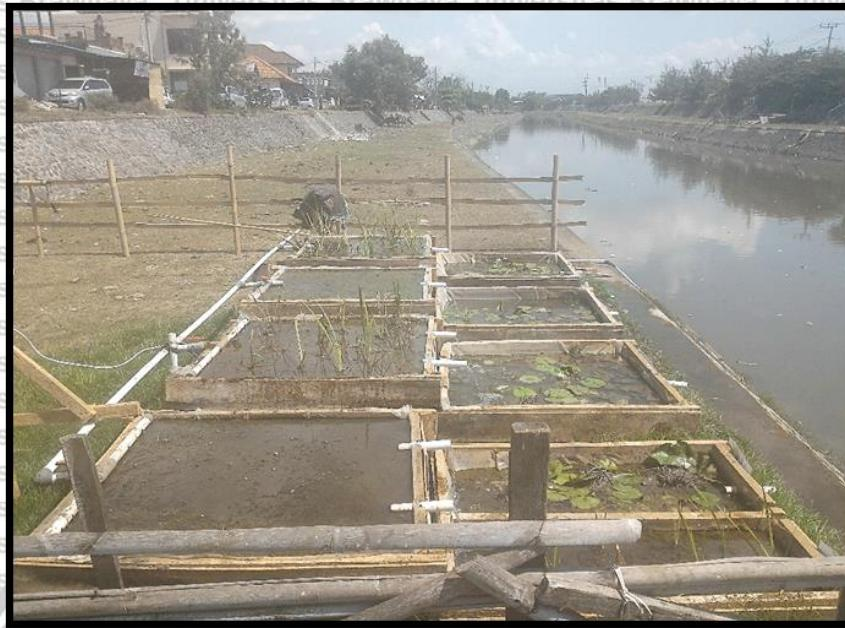
**Gambar 4.5. Model Wetland Test Kombinasi Surface dan Subsurface**
