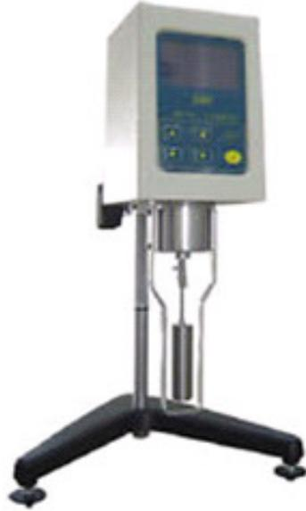
Gambar 4-3 Viskometer NDJ 8 S
