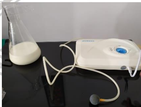
Figure 3. Ozone generator preparation
