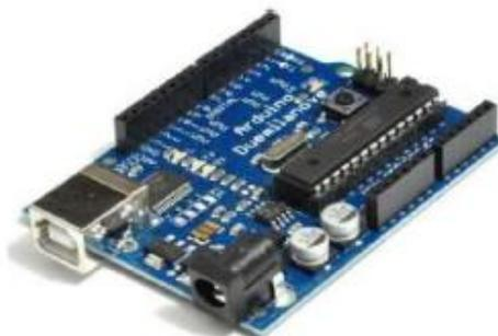
**Gambar 2.5 Arduino UNO Board**
