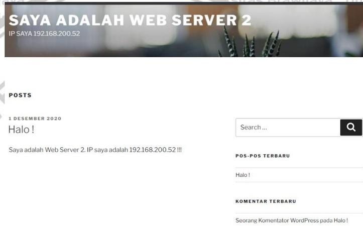
**Gambar 6.12 Mengakses Alamat IP Virtual Keepalived Setelah Service Keepalived Pada Web Server 1 Mati**
