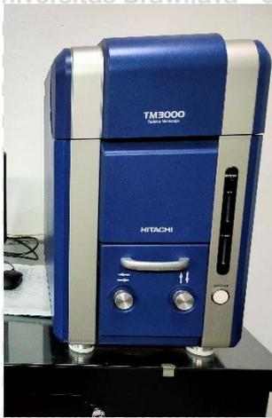
*Gambar 3.7 Scanning Electron Microscope*
