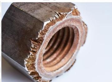
Gambar 2.20 Crevice Corrosion
