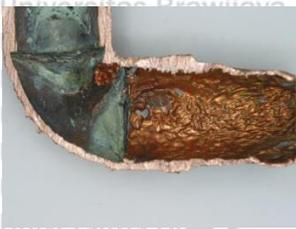
Gambar 2.24 Errosion Corrosion
