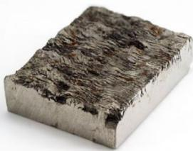
Gambar 2.23 *Intergranular corrosion*
