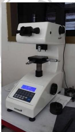
Gambar 3.6 Microvickers EW-412AAT Hardness Testing Machine
