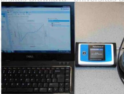
Gambar 3.9 Potentiostat/Galvanostat Instrument
