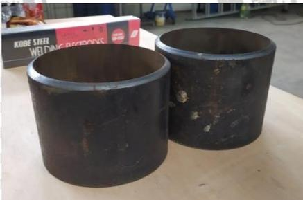
Gambar 3.11 Spesimen ASTM A106 grade B
