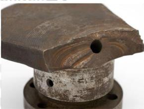
Gambar 2.25 Fatigue Corrosion
