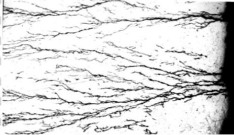
Gambar 2.5 *Stress corrosion cracking*
