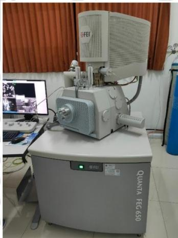
Gambar 3.9 FE-SEM Quanta FEG 650
