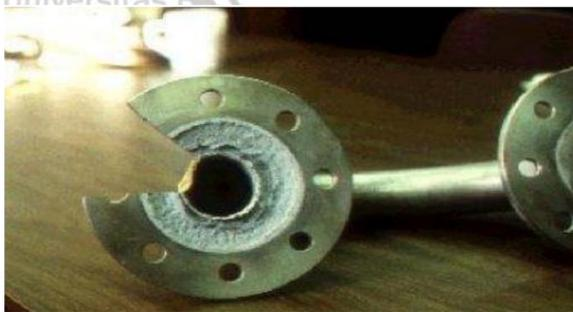
Gambar 2.8 Crivice corrosion
