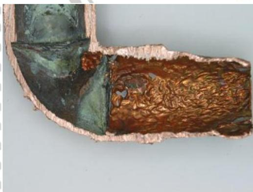
Gambar 2.6 *Errosion corrosion*
