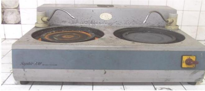
Gambar 3.3 Centrifugal sand paper machine
