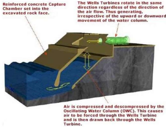
Gambar 3. Oscillating Water Column model Limpet (Drew, et al., 2009)
