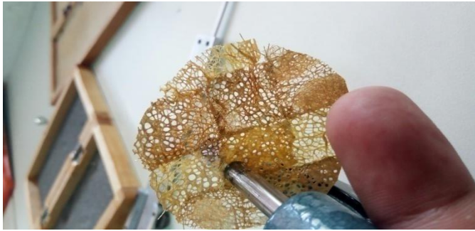
Gambar 3.4 Pengukuran Ketebalan filter
