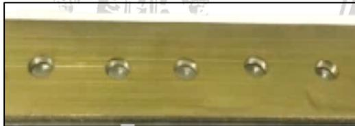
**Gambar 4.1** *Master Cast Logam (Mould)*
