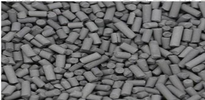
Gambar 2.4 *Extruded activated carbon*
