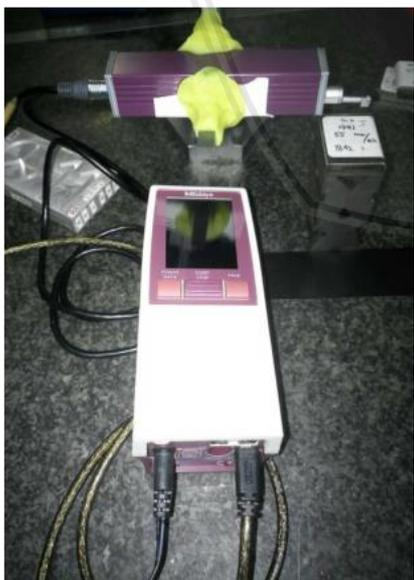
Gambar 3.8 *Surface roughness tester*
