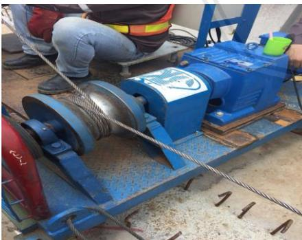
Gambar 4.12 Mesin *Power Winch*
