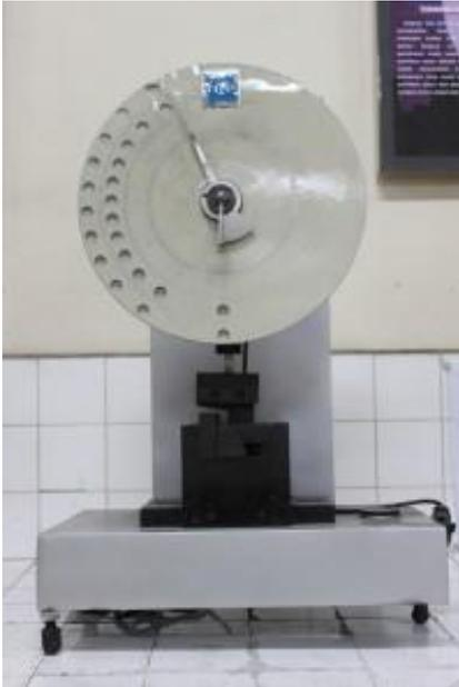
*Gambar 2.6 Plastics Charpy Impact Test Machine*
