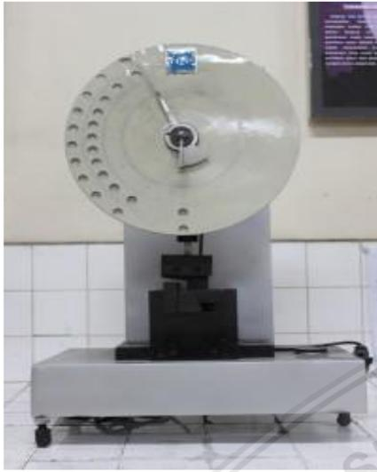
*Gambar 3.8 Plastics Charpy Impact Test Machine*
