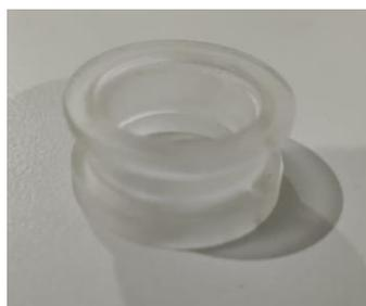
Gambar 5.7 Hasil cetak *chamber liquid impedance analyser*
