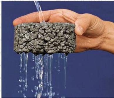
Gambar 2.1 *Pervious Concrete*
