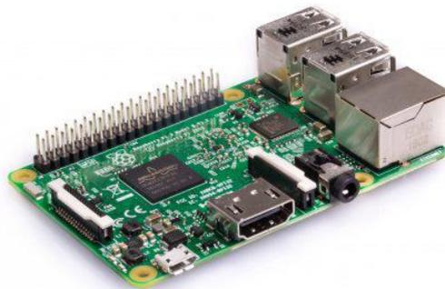
Gambar 2.19 Raspberry Pi 3 Model B
