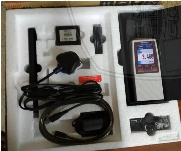
Gambar 3.6 Surface roughness tester
