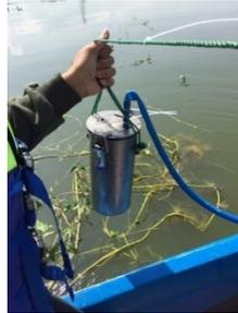
Gambar 3. Alat *Vertical Water Sampler*
