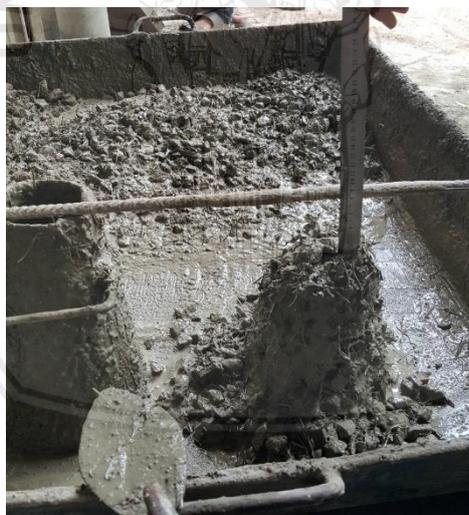
**Gambar 4.1** Proses Uji *Slump*
