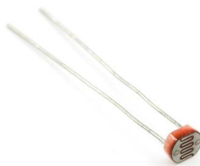
Gambar 2.4 Sensor Cahaya Photoresistor LDR GL5528
