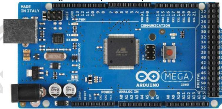
**Gambar 2.6** Arduino Mega 2560
