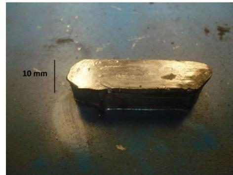
Gambar 4.18 Aluminium Hasil proses ECAP
