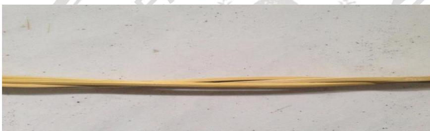
Gambar 4. 6 Pola Bambu Pilin
