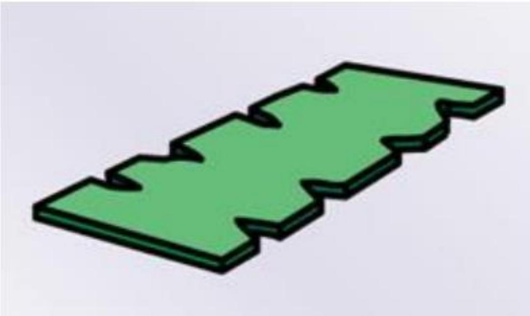
Gambar 2.21 Side Cracks
