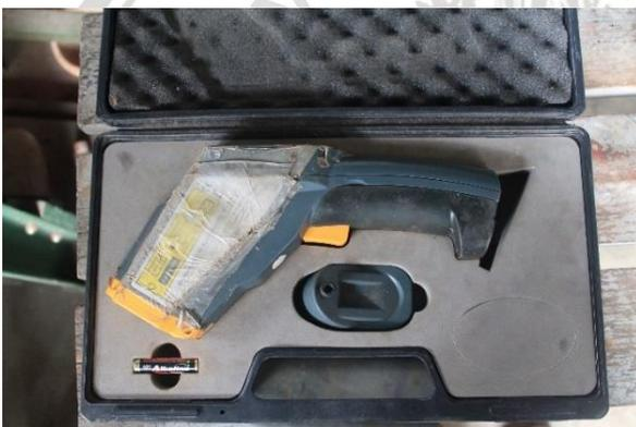
Gambar 3.3 Thermogun type TM 969
